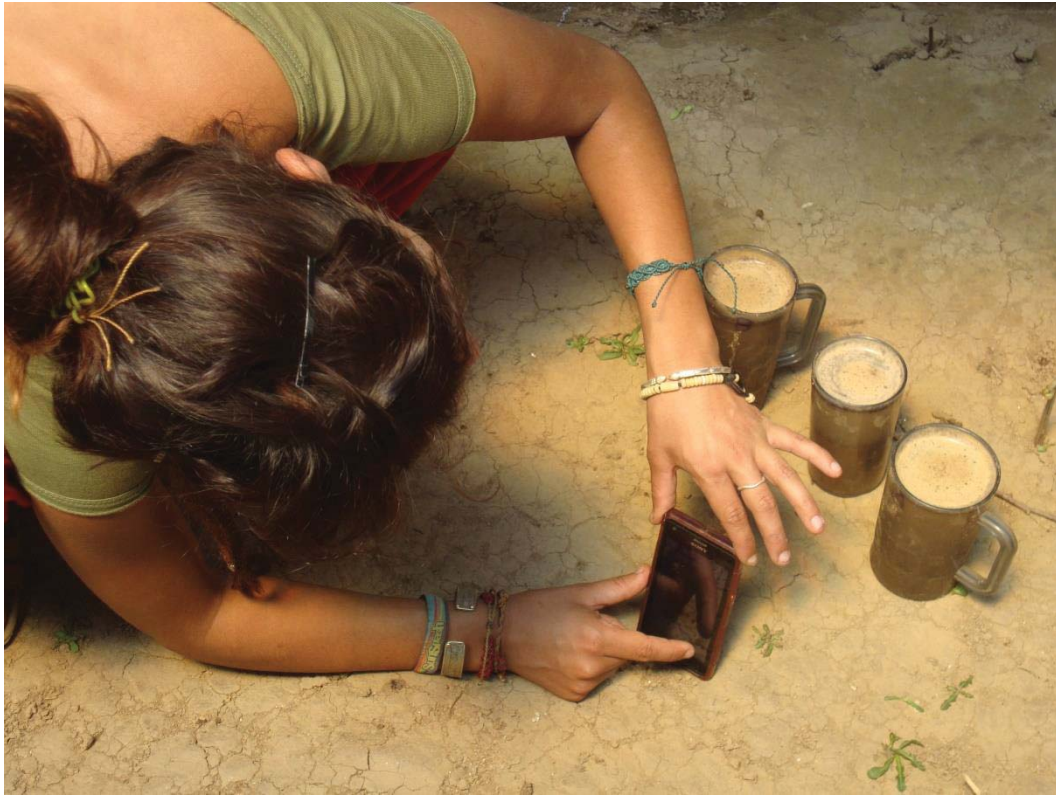
Figure 8: Three glasses of soil samples with water for soil size analysis.
